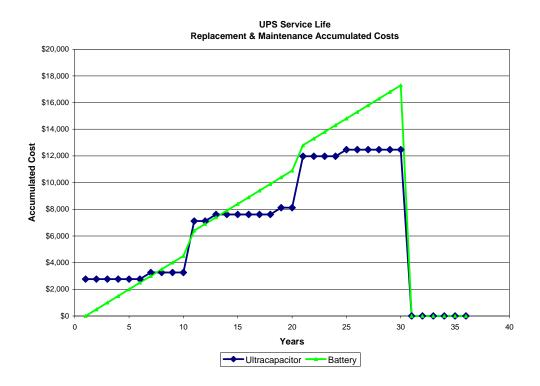
Figure 2: Accumulated cost of best case battery life vs. expected ultracapacitor life
