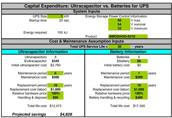
Figure 1: Best case battery life vs. expected ultracapacitor life
