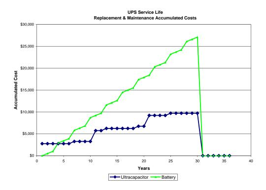
Figure 4: Accumulated cost of worst case battery life vs. expected ultracapacitor life
