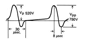
The Vrms voltage derived from the peak voltage shall always be less than the nominal AC voltage rating of the capacitor. Other restrictions may apply.
