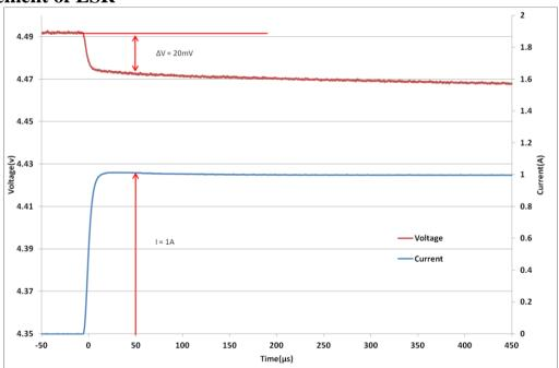
Fig 3: Measurement of ESR for a GS208
