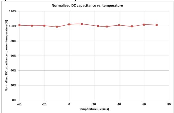
Figure 6: Capacitance change with temperature
