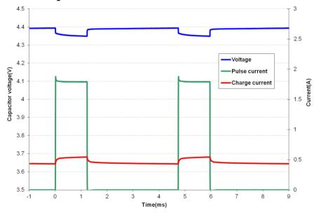
Fig 5 shows that the GS208 supercapacitor does an excellent job supporting a GPRS class 10 pulse train, drawing 1.8A for 1.1ms at 25% duty cycle. The source is current limited to 0.6A and the supercapacitor provides the 1.2A difference to achieve the peak current. At first glance the freq response of Fig 8 indicates the supercapacacitor would not support a 1ms pulse, but the Ceff of 58.5mF coupled with the low ESR supports this pulse train with only ~45mV droop in the supply rail.
