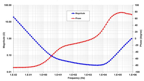
Fig 8: Frequency Response of Impedance (biased at 5V with a 50mV test signal)
