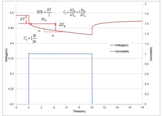
Figure 1: Effective capacitance, instantaneous capacitance and ESR for a GS206
