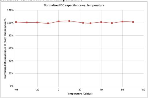
Figure 6: Capacitance change with temperature
