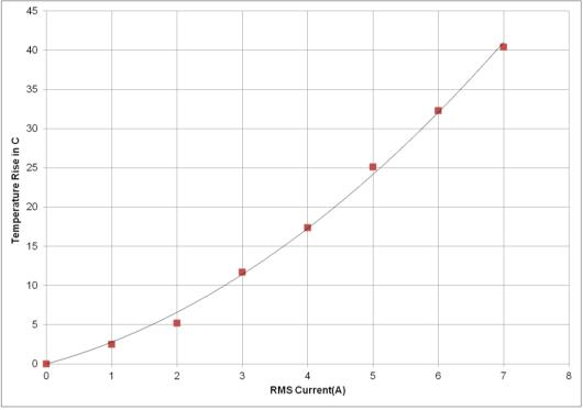
Fig 12: Temperature rise in GS206 with RMS current
