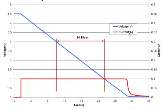
Fig 2: Measurement of DC Capacitance for a GS206
