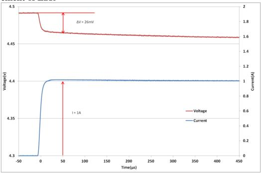
Fig 3: Measurement of ESR for a GS206
