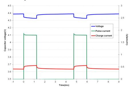
Fig 5 shows that the GS206 supercapacitor does an excellent job supporting a GPRS class 10 pulse train, drawing 1.8A for 1.1ms at 25% duty cycle. The source is current limited to 0.6A and the supercapacitor provides the 1.2A difference to achieve the peak current. At first glance the freq response of Fig 8 indicates the supercapacacitor would not support a 1.1ms pulse, but the Ceff of 122mF coupled with the low ESR supports this pulse train with only ~60mV droop in the supply rail.
