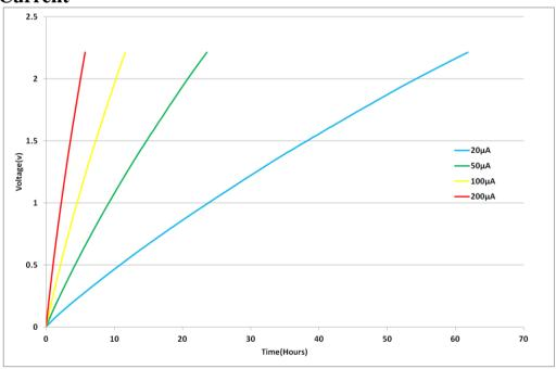
Fig 11: Charging a GS106 with low current
