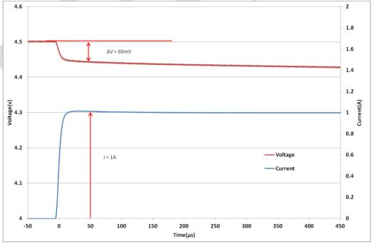
Fig 3: Measurement of ESR for a GA230
