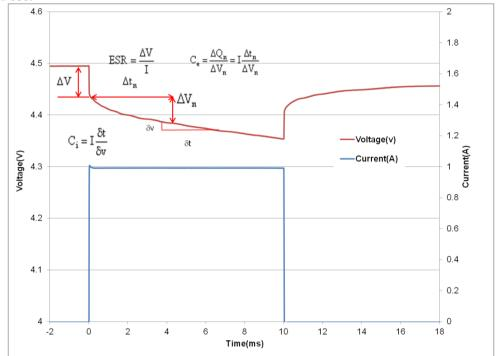
Figure 1: Effective capacitance, instantaneous capacitance and ESR for a GA230
