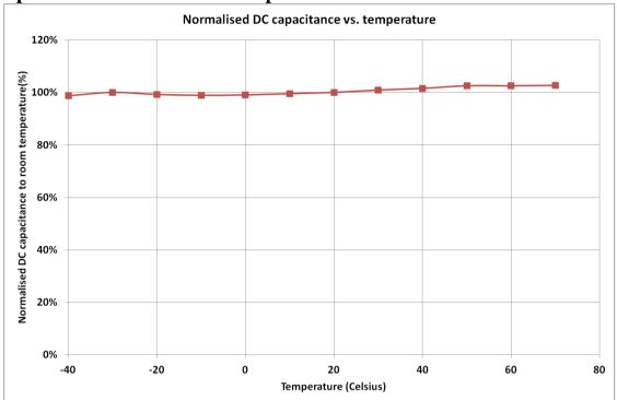
Figure 6: Capacitance change with temperature
