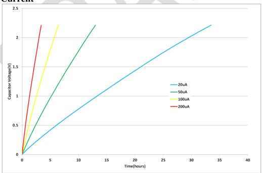
Fig 11: Charging an GA130 with low current
