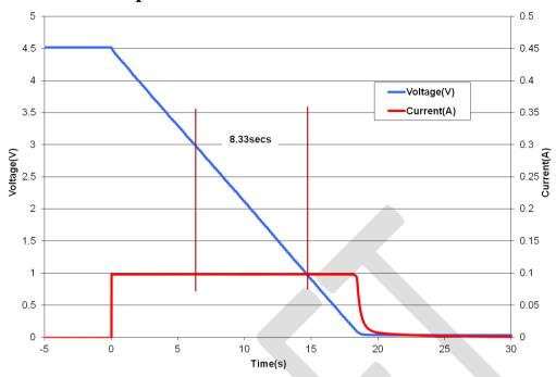
Fig 2: Measurement of DC Capacitance for a GA230
