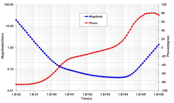
Fig 8: Frequency Response of Impedance (biased at 2.7V with a 50mV test signal)
