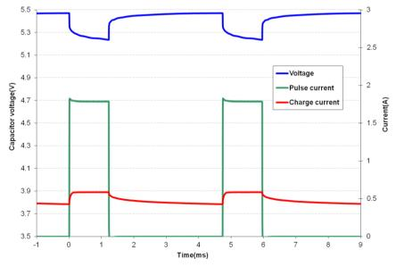
Fig 5 shows that the HW201 supercapacitor does an excellent job supporting a GPRS class 10 pulse train, drawing 1.8A for 1.1ms at 25% duty cycle. The source is current limited to 0.6A and the supercapacitor provides the 1.2A difference to achieve the peak current. At first glance the freq response of Fig 8 indicates the supercapacacitor would not support a 1ms pulse, but the Ceff of 34.2mF coupled with the low ESR supports this pulse train with only ~230mV droop in the supply rail.
