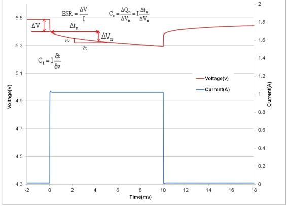
Figure 1: Effective capacitance, instantaneous capacitance and ESR for an HW201
