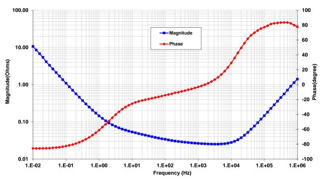
Fig 8: Frequency Response of Impedance (biased at 2.7V with a 50mV test signal)
