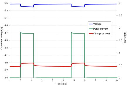
Fig 5 shows that the HS206 supercapacitor does an excellent job supporting a GPRS class 10 pulse train, drawing 1.8A for 1.1ms at 25% duty cycle. The source is current limited to 0.6A and the supercapacitor provides the 1.2A difference to achieve the peak current. At first glance the freq response of Fig 8 indicates the supercapacacitor would not support a 1ms pulse, but the Ceff of 65mF coupled with the low ESR supports this pulse train with only ~80mV droop in the supply rail.
