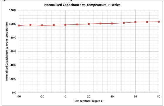
Figure 6: Capacitance change with temperature
