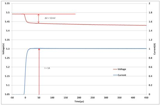
Fig 3: Measurement of ESR for an HS206
