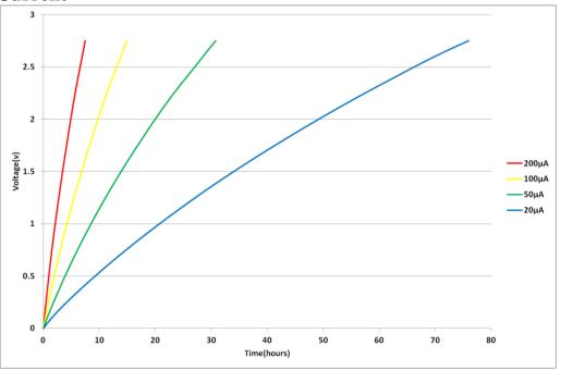
Fig 11: Charging an HS106 with low current
