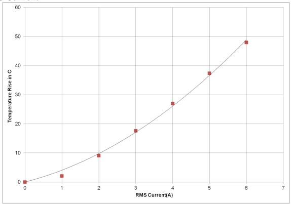
Fig 12: Temperature rise in HS206 with RMS current
