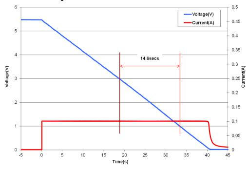
Fig 2: Measurement of DC Capacitance for an HS206
