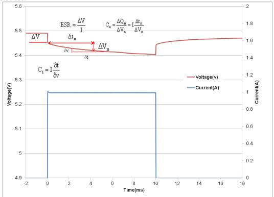
Figure 1: Effective capacitance, instantaneous capacitance and ESR for an HS208
