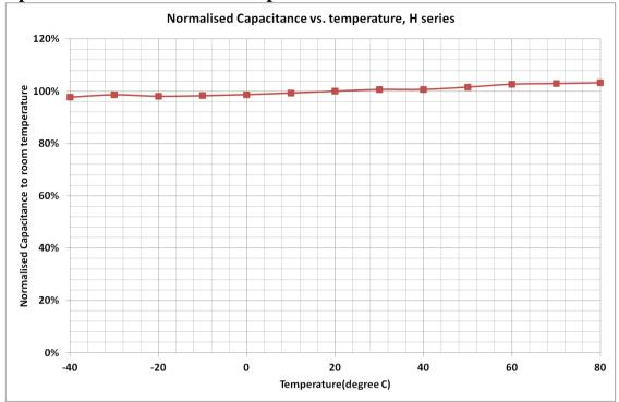
Figure 6: Capacitance change with temperature
