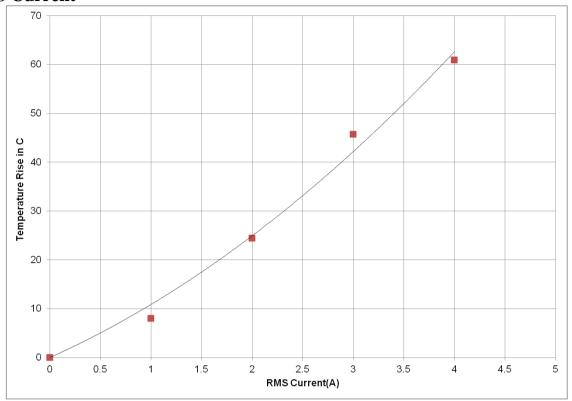
Fig 12: Temperature rise in HA230 with RMS current
