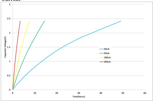
Fig 11: Charging an HA130 with low current
