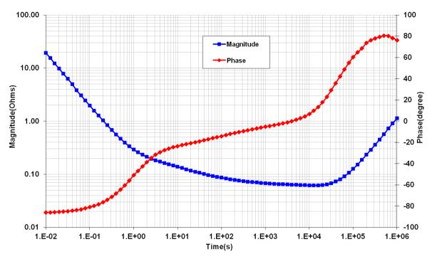
Fig 8: Frequency Response of Impedance (biased at 2.5V with a 50mV test signal)
