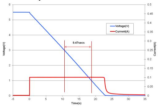
Fig 2: Measurement of DC Capacitance for an HA230
