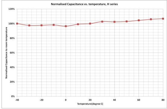
Figure 6: Capacitance change with temperature
