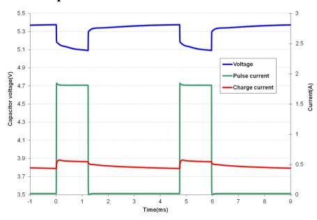
Fig 5 shows that the HA230 supercapacitor does an excellent job supporting a GPRS class 10 pulse train, drawing 1.8A for 1.1ms at 25% duty cycle. The source is current limited to 0.6A and the supercapacitor provides the 1.2A difference to achieve the peak current. At first glance the freq response of Fig 8 indicates the supercapacacitor would not support a 1ms pulse, but the Ceff of 26mF coupled with the low ESR supports this pulse train with only ~280mV droop in the supply rail.
