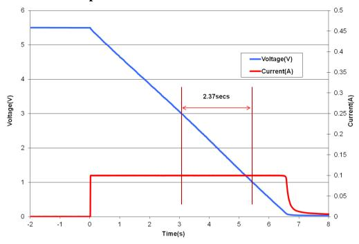
Fig 2: Measurement of DC Capacitance for an HA202
