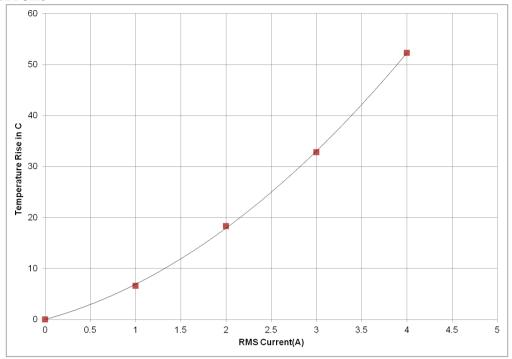
Fig 12: Temperature rise in HA202 with RMS current
