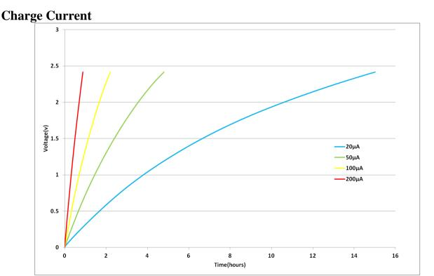
Fig 11: Charging an HA102 with low current
