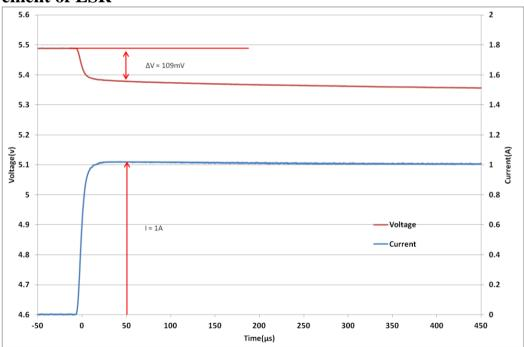
Fig 3: Measurement of ESR for an HA202
