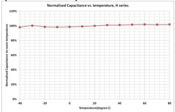
Figure 6: Capacitance change with temperature
