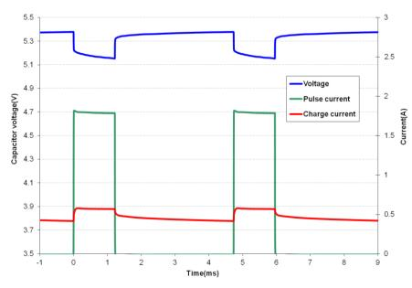
Fig 5 shows that the HA202 supercapacitor does an excellent job supporting a GPRS class 10 pulse train, drawing 1.8A for 1.1ms at 25% duty cycle. The source is current limited to 0.6A and the supercapacitor provides the 1.2A difference to achieve the peak current. At first glance the freq response of Fig 8 indicates the supercapacacitor would not support a 1ms pulse, but the Ceff of 22.8mF coupled with the low ESR supports this pulse train with only ~220mV droop in the supply rail.
