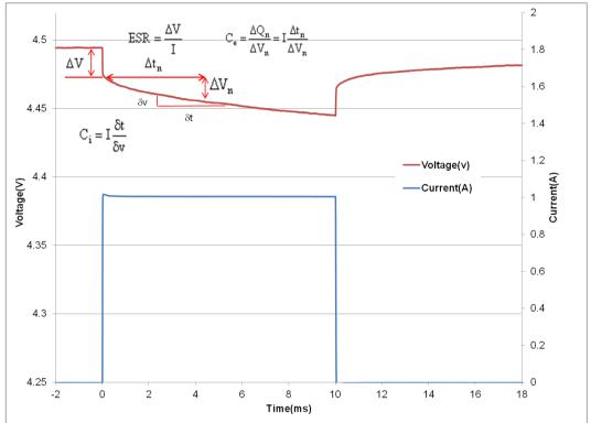
Figure 1: Effective capacitance, instantaneous capacitance and ESR for a GS230
