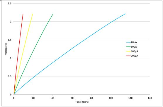
Fig 11: Charging a GS130 with low current
