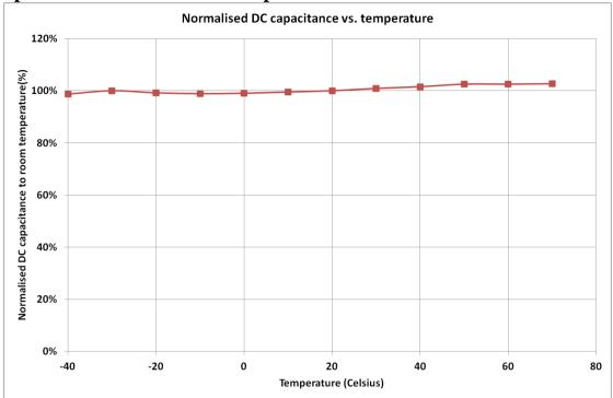
Figure 6: Capacitance change with temperature
