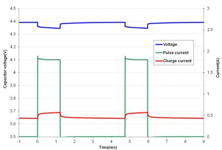
Fig 5 shows that the GS230 supercapacitor does an excellent job supporting a GPRS class 10 pulse train, drawing 1.8A for 1.1ms at 25% duty cycle. The source is current limited to 0.6A and the supercapacitor provides the 1.2A difference to achieve the peak current. At first glance the freq response of Fig 8 indicates the supercapacacitor would not support a 1ms pulse, but the Ceff of 132mF coupled with the low ESR supports this pulse train with only ~50mV droop in the supply rail.
