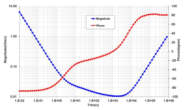
Fig 8: Frequency Response of Impedance (biased at 2.3V with a 50mV test signal)
