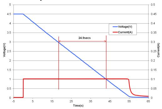
Fig 2: Measurement of DC Capacitance for a GS230
