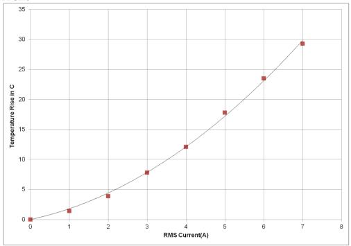
Fig 12: Temperature rise in GS230 with RMS current
