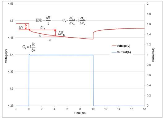
Figure 1: Effective capacitance, instantaneous capacitance and ESR for a GS208
