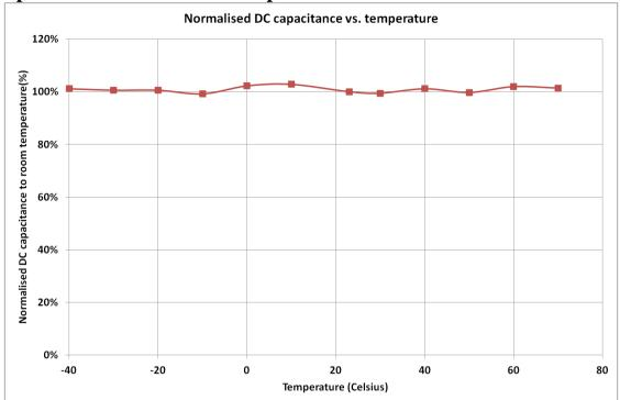
Figure 6: Capacitance change with temperature
