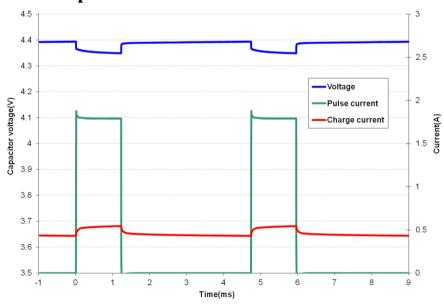
Fig 5 shows that the GS208 supercapacitor does an excellent job supporting a GPRS class 10 pulse train, drawing 1.8A for 1.1ms at 25% duty cycle. The source is current limited to 0.6A and the supercapacitor provides the 1.2A difference to achieve the peak current. At first glance the freq response of Fig 8 indicates the supercapacacitor would not support a 1ms pulse, but the Ceff of 58.5mF coupled with the low ESR supports this pulse train with only ~45mV droop in the supply rail.
