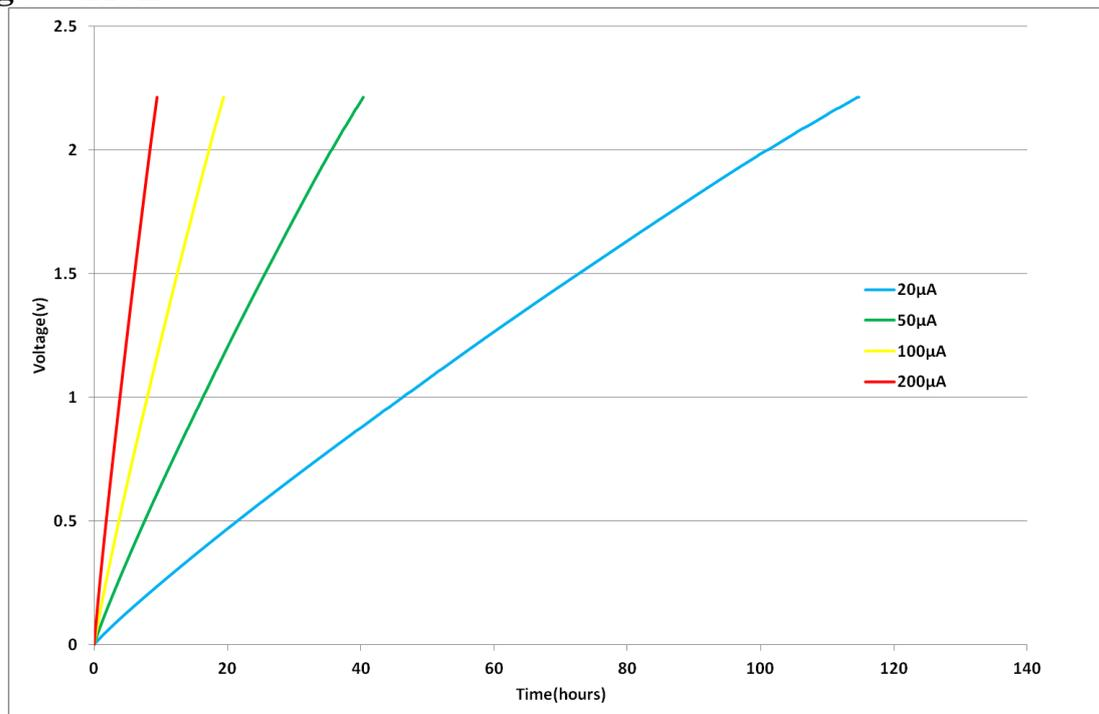
**Fig 11: Charging a GS130 with low current**
