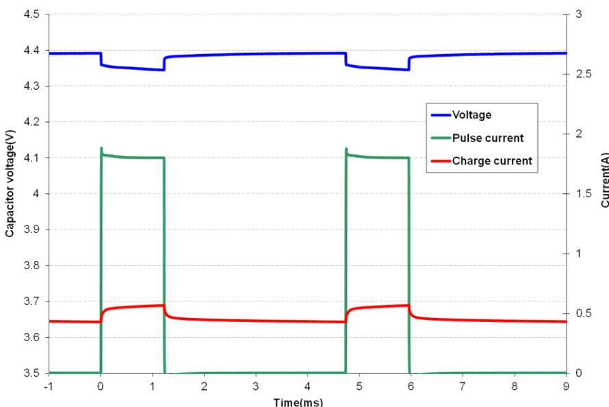
Fig 5 shows that the GS230 supercapacitor does an excellent job supporting a GPRS class 10 pulse train, drawing 1.8A for 1.1ms at 25% duty cycle. The source is current limited to 0.6A and the supercapacitor provides the 1.2A difference to achieve the peak current. At first glance the freq response of Fig 8 indicates the supercapacitor would not support a 1ms pulse, but the  $C_{eff}$  of 132mF coupled with the low ESR supports this pulse train with only ~50mV droop in the supply rail.
