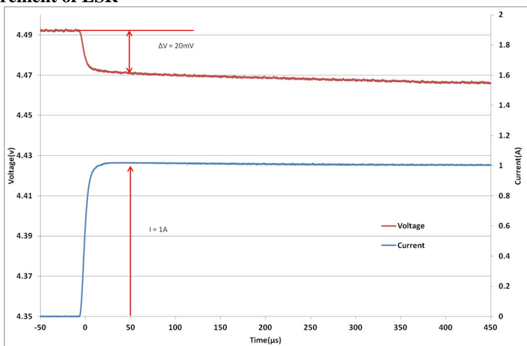
**Fig 3: Measurement of ESR for a GS230**
